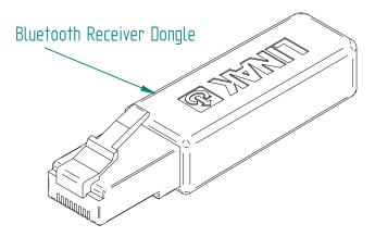
Make sure dongle is placed outside of cabinet to ensure good connection to the Bluetooth remote transmitter (Extension cable supplied with receiver).
